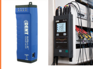
Power Meter with Data Logger and Various CT sizes
