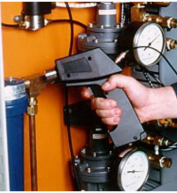
Ultrasonic Leak Detector for CDA and Steam Traps
