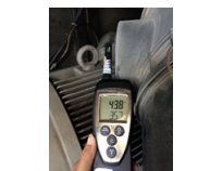
Inlet Air Conditions Measurement
